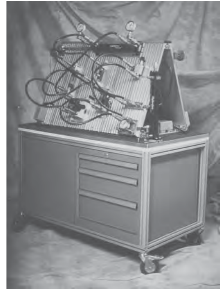
Profile 16x160 used in pneumatic training station (photo courtesy of National Technology Transfer, Inc.)
